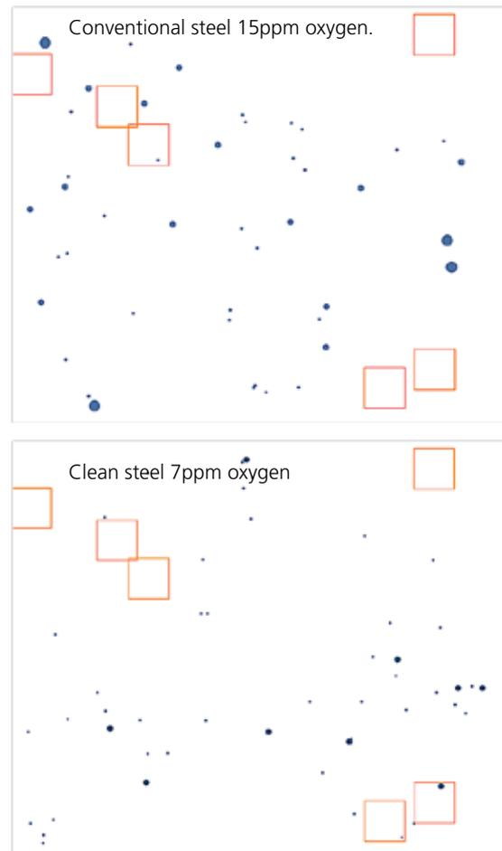
*Fig 4 – A specific issue with LOM is the small sample size as shown in this schematic illustration (not to scale). Normal procedure is to examine 6 samples. But their small size does not represent the true size and distribution of inclusions. In this particular case it is even possible to obtain the false impression that standard steel (4a) has fewer and smaller inclusions than a clean steel (4b).*
