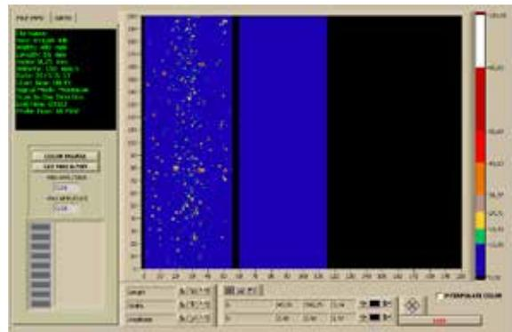
Fig 11 – Ultrasonic C-Scan (10MHz), Steel A (left) and Steel B(right)
