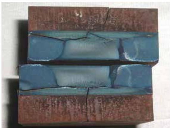
Fig 8 – Blue fracture test showing no indication of any inclusion
