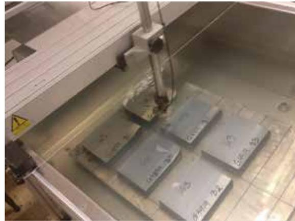
Fig 6 – immersed ultrasonic testing at Ovako
