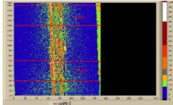
Fig 9 - Ultrasonic scan showing the positions where blue fracture specimens were selected.
